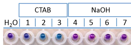
Figure 28: Influence of CTAB and NaOH on the colour of LAMP reaction solutions with HNB. Two \mu l of the test solution was added to 23 \mu l of LAMP reaction solution. Test solution no. 1 = CTAB diluted 1:100 with water; 2 = CTAB diluted 1:10 with water; 3 = CTAB undiluted; 4 = NaOH (0.5 M) diluted 1:10 with water; 5 = NaOH (0.5 M) diluted 1:10 with Tris-HCl (pH 8.8; 100 mM); 6 = NaOH (0.5 M) diluted 1:100 with water; 7 = NaOH (0.5 M) diluted 1:100 with Tris-HCl (pH 8.8; 100 mM).
