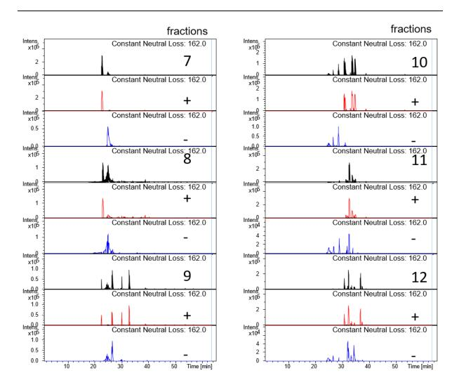
**Figure S5.** LC-MS analysis of selected fractions (7-12) of the tobacco extract. Different putative hexosides (neutral loss of 162) can be inferred from the neutral loss experiments in the positive and negative mode.
