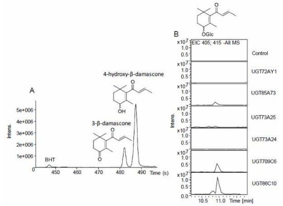
**Figure 21.** LC-MS analysis of monglucosides of 4-hydroxy- $\beta$ -damascone produced by selected UGTs (right B), and GC-MS of the substrate mix (left, A) obtained by whole-cell P450 monooxygenase biotransformation. BHT butylated hydroxytoluene, LC-MS ion traces at *m/z* 405 and 415 show 4-OH- $\beta$ -damascone glucoside.
